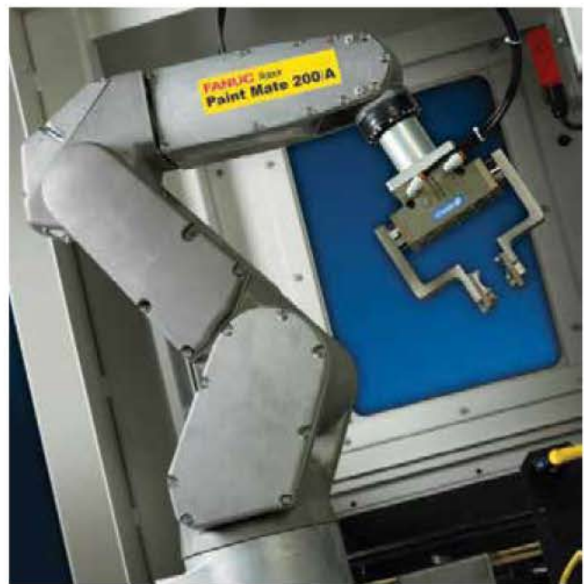
Class 1 Division 1 hazardous approval ratings enables the Paint Mate robot to be used for handling applications in explosive and extreme environments
